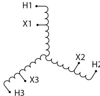
Three Phase Autotransformer with a capacity of 3kVA, transforming 440Y Volts to 400Y Volts
