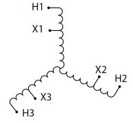
Three Phase Autotransformer with a capacity of 3kVA, transforming 440Y Volts to 120Y Volts
