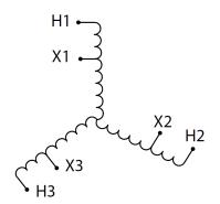
Three Phase Autotransformer with a capacity of 3kVA, transforming 240Y Volts to 347Y Volts
