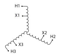
Three Phase Autotransformer with a capacity of 3kVA, transforming 240Y Volts to 200Y Volts
