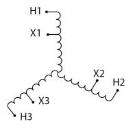
Three Phase Autotransformer with a capacity of 30kVA, transforming 460Y Volts to 220Y Volts
