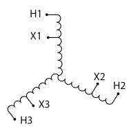
Three Phase Autotransformer with a capacity of 30kVA, transforming 416Y Volts to 277Y Volts
