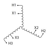
Three Phase Autotransformer with a capacity of 30kVA, transforming 400Y Volts to 115Y Volts
