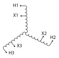
Three Phase Autotransformer with a capacity of 30kVA, transforming 400Y Volts to 110Y Volts
