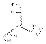
Three Phase Autotransformer with a capacity of 30kVA, transforming 347Y Volts to 575Y Volts
