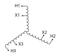
Three Phase Autotransformer with a capacity of 30kVA, transforming 347Y Volts to 240Y Volts
