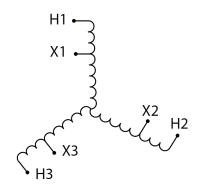
Three Phase Autotransformer with a capacity of 30kVA, transforming 347Y Volts to 240Y Volts
