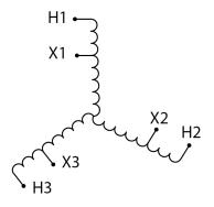
Three Phase Autotransformer with a capacity of 30kVA, transforming 277Y Volts to 600Y Volts
