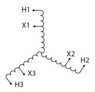
Three Phase Autotransformer with a capacity of 30kVA, transforming 220Y Volts to 110Y Volts
