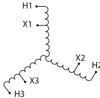
Three Phase Autotransformer with a capacity of 30kVA, transforming 200Y Volts to 460Y Volts
