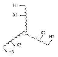
Three Phase Autotransformer with a capacity of 30kVA, transforming 110Y Volts to 460Y Volts
