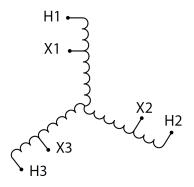
Three Phase Autotransformer with a capacity of 30kVA, transforming 110Y Volts to 440Y Volts
