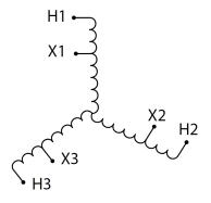
Three Phase Autotransformer with a capacity of 30kVA, transforming 110Y Volts to 240Y Volts
