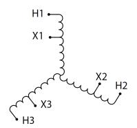
Three Phase Autotransformer with a capacity of 15kVA, transforming 575Y Volts to 347Y Volts
