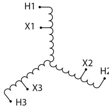
Three Phase Autotransformer with a capacity of 15kVA, transforming 550Y Volts to 380Y Volts
