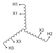
Three Phase Autotransformer with a capacity of 15kVA, transforming 550Y Volts to 115Y Volts
