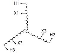
Three Phase Autotransformer with a capacity of 15kVA, transforming 440Y Volts to 575Y Volts
