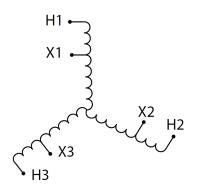
Three Phase Autotransformer with a capacity of 15kVA, transforming 415Y Volts to 277Y Volts
