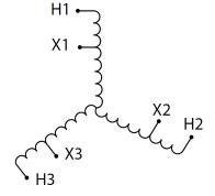
Three Phase Autotransformer with a capacity of 15kVA, transforming 415Y Volts to 230Y Volts
