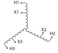
Three Phase Autotransformer with a capacity of 15kVA, transforming 415Y Volts to 200Y Volts
