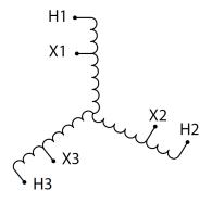
Three Phase Autotransformer with a capacity of 15kVA, transforming 380Y Volts to 115Y Volts
