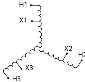
Three Phase Autotransformer with a capacity of 15kVA, transforming 347Y Volts to 277Y Volts
