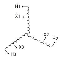
Three Phase Autotransformer with a capacity of 15kVA, transforming 277Y Volts to 550Y Volts
