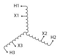
Three Phase Autotransformer with a capacity of 15kVA, transforming 230Y Volts to 240Y Volts
