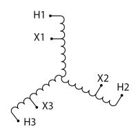
Three Phase Autotransformer with a capacity of 15kVA, transforming 230Y Volts to 115Y Volts
