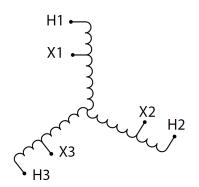
Three Phase Autotransformer with a capacity of 15kVA, transforming 220Y Volts to 600Y Volts
