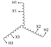
Three Phase Autotransformer with a capacity of 15kVA, transforming 208Y Volts to 115Y Volts
