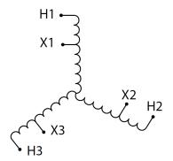
Three Phase Autotransformer with a capacity of 15kVA, transforming 120Y Volts to 460Y Volts
