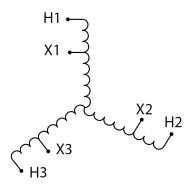
Three Phase Autotransformer with a capacity of 15kVA, transforming 115Y Volts to 380Y Volts
