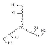
Three Phase Autotransformer with a capacity of 15kVA, transforming 115Y Volts to 120Y Volts
