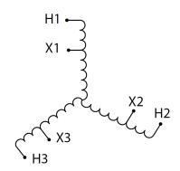
Three Phase Autotransformer with a capacity of 15kVA, transforming 115Y Volts to 110Y Volts
