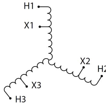
Three Phase Autotransformer with a capacity of 150kVA, transforming 416Y Volts to 347Y Volts
