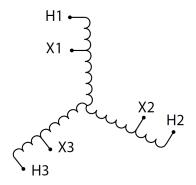
Three Phase Autotransformer with a capacity of 150kVA, transforming 115Y Volts to 220Y Volts
