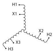
Three Phase Autotransformer with a capacity of 1500kVA, transforming 550Y Volts to 460Y Volts
