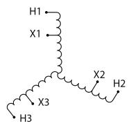
Three Phase Autotransformer with a capacity of 1500kVA, transforming 480Y Volts to 575Y Volts
