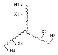
Three Phase Autotransformer with a capacity of 1500kVA, transforming 460Y Volts to 600Y Volts
