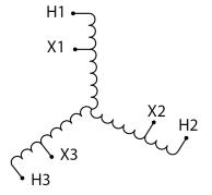
Three Phase Autotransformer with a capacity of 112.5kVA, transforming 600Y Volts to 115Y Volts
