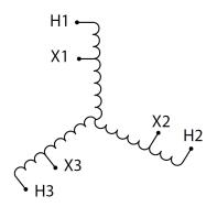
Three Phase Autotransformer with a capacity of 112.5kVA, transforming 240Y Volts to 110Y Volts
