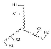
Three Phase Autotransformer with a capacity of 112.5kVA, transforming 220Y Volts to 110Y Volts
