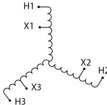
Three Phase Autotransformer with a capacity of 112.5kVA, transforming 120Y Volts to 277Y Volts
