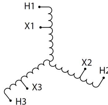
Three Phase Autotransformer with a capacity of 112.5kVA, transforming 110Y Volts to 415Y Volts
