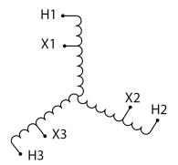
Three Phase Autotransformer with a capacity of 112.5kVA, transforming 110Y Volts to 347Y Volts
