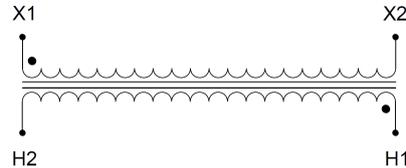
Single Phase Control Transformer with a capacity of 350VA, transforming 600 Volts to 115 Volts
