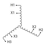
Three Phase Autotransformer with a capacity of 3kVA, transforming 115Y Volts to 220Y Volts
