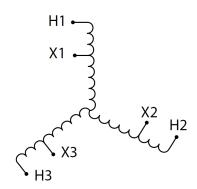
Three Phase Autotransformer with a capacity of 3kVA, transforming 115Y Volts to 550Y Volts
