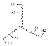
Three Phase Autotransformer with a capacity of 75kVA, transforming 120Y Volts to 416Y Volts
